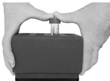
Figure 5: Insert a tall cylindrical object into an empty tube well
