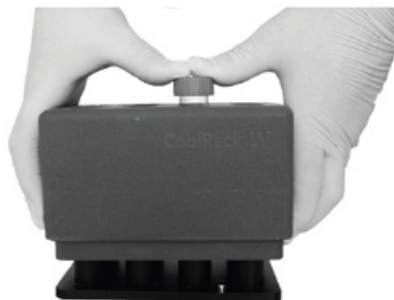
Figure 6: Push the cylindrical object down while pulling the external housing from the base to release the magnets. Pull the housing off the tube wells.
