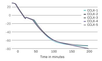
Conclusion: Cell Freezing container showed identical cooling profiles and phase transition over five consecutive freeze cycles.
