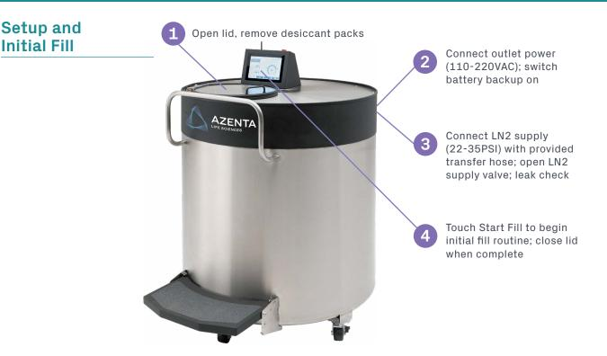
The initial fill can take 1-2 hours. When complete, normal controller operation will maintain LN2 levels while monitoring and logging storage conditions. Allow the freezer to cool for 48 hours before introducing samples. Routinely verify freezer status and ensure sufficient LN2 supply.
