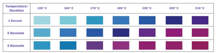
**Note:** This colour chart is just an example based on the results of the tests performed in our laboratories. Before using the Thermal Test Film, please create a similar chart that is based on your actual measurement conditions.
