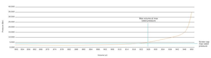
Chart Showing Fill Volume vs Pressure at -80°C Azenta "1.4ml" Internal Thread Screw Cap Tube
